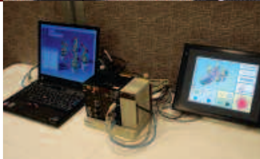
Demonstration machine integrating OMRON PLC set-up and DELMIA Automation
